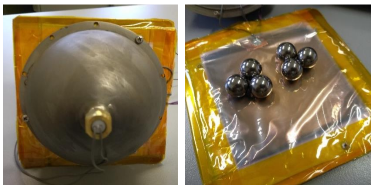
Figure 1. Photography of the floating buoy-based triboelectric nanogenerator.
