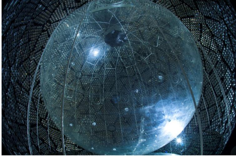
**Figure 1.** The SNO+ detector. The outer 18 m diameter geodesic structure holds ~9300 inward-facing PMTs within a volume of highly purified water. The scintillator will fill the inner 12 m diameter acrylic vessel.
